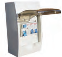
MCU2516 Mains consumer unit fitted with a 25 A / 30mA RCCB residual current device and 2 MCB's 1 x 6 amp 1 x 10 amp. Dimensions 200 x 112 x 90mm
