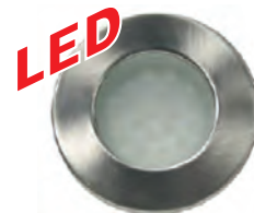
NEW LED42FSRMN LED Fixed recessed or surface mount with surround supplied. Led downlight of superb quality with 42 LED's for high output. Connect to 12volt DC. 2.5w Size 70mm Ø x 17mm recessed or 32mm High surface mounted.
