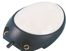
L834 Automatic Cupboard light Nice oval styled slim profile push switch light. Mount on cupboard frame with door in contact with spring loaded push switch. As you open door light will come on. Turns off when door closed. Fitted 10w filament bulb. Size 105L x 85W x 40H. Colour: Brown.
