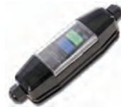
MLLRCD In Line 16 amp mobile RCD Ideal for tenting or garden power products, Wired between the appliance & mains plug, Reset & test light facility, Trip speed: 30mS, Can be used in damp & wet conditions
