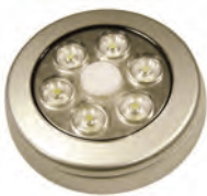
LED101SG 6 SUPERBRIGHT LED Recessed or surface mount down lighter. Sizes: Ø 75 x 8mm recessed requires 56mm hole. Surface mounted 78mm Ø x 19mm H. With centre illuminated blue switch.
