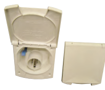
Mains inlet socket styled to match F30/1 water filler (page 19). Sizes 137mm High x 122mm Wide. Cut out oval 90mm H x 85mm W. MIF30 White mains inlet MIF31 Black mains inlet
