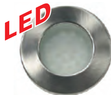
NEW LED30FSRMN LED Fixed recessed or surface mount with surround supplied. Led downlight of superb quality with 30 LED's for high output. Connect to 12volt DC. 1.8w Size 70mm Ø x 17mm recessed or 32mm High surface mounted.
